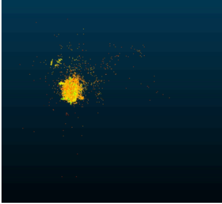
Figure 4.3: Point cloud reconstruction using 13 cameras and 21 frames per camera.
