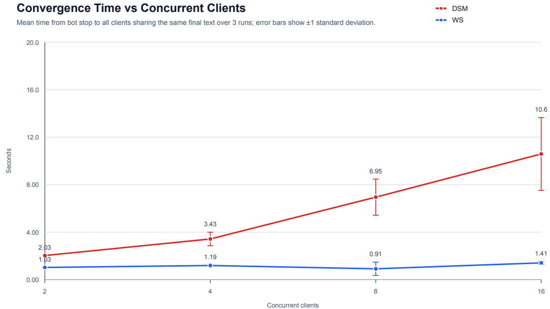
Figure 5.7: Time from bot stop until all clients share the same final text. Error bars show \pm 1 standard deviation over three runs.
