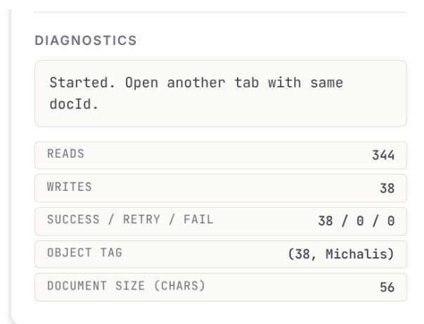
Figure 4.5: Runtime diagnostics panel of the collaborative editing prototype
