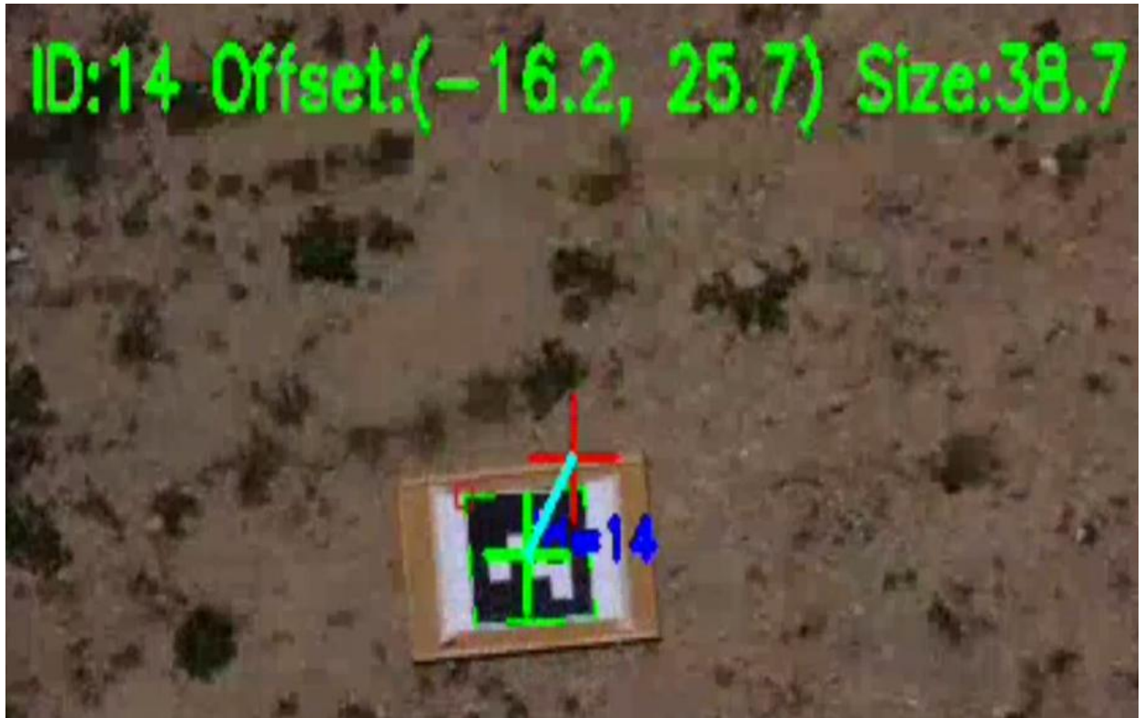
Figure 3: Example of ArUco marker detection in an image frame using OpenCV, showing the detected marker boundary, decoded marker ID, and geometric reference used for localization.
