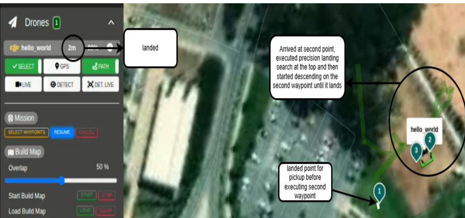
Figure 12: Showing landing on few waypoints and the precision landing searching for the ArUco marker that made the UAV move left and right accordingly.
