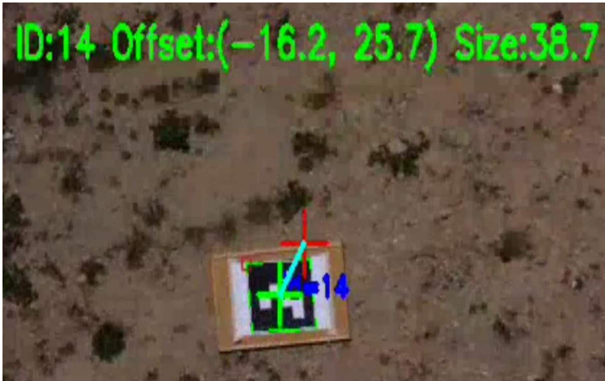
Figure 17: Live onboard ArUco detection that needs to be at 6 meters due to image resizing and quality.
