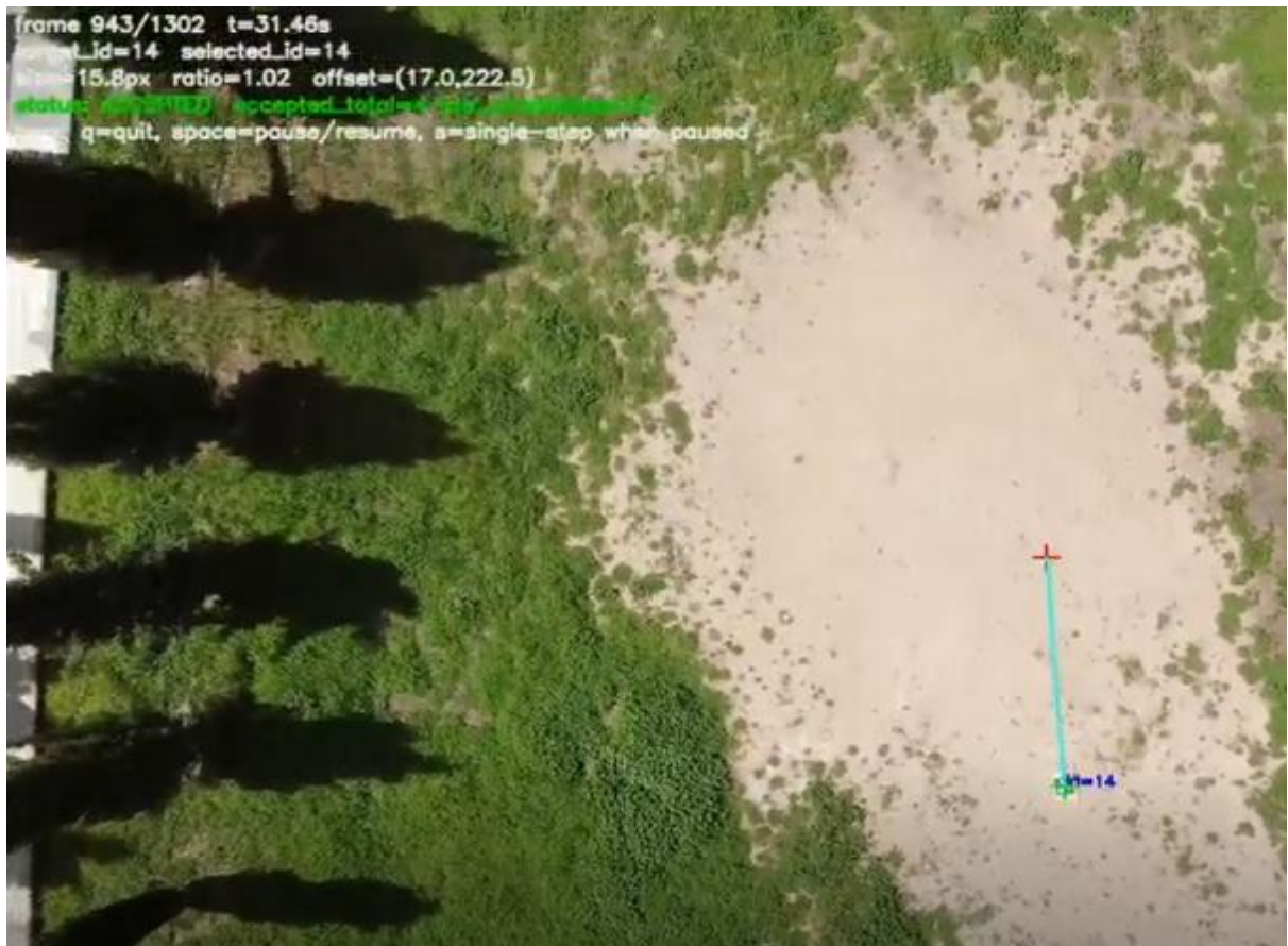
Figure 18: Recorder Video detection of ArUco marker (ID=14) with better quality and greater distance.
