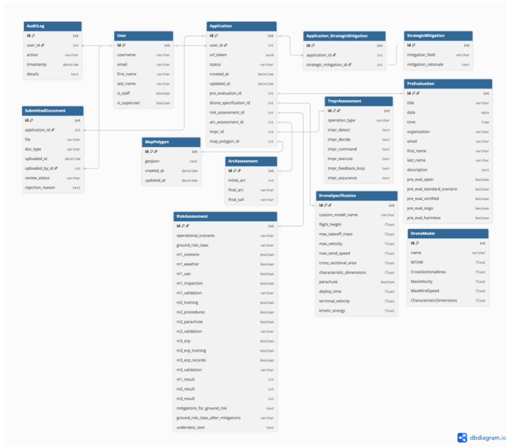
Figure 4.2: Entity-relationship diagram for the SORA 2.0 application workflow
