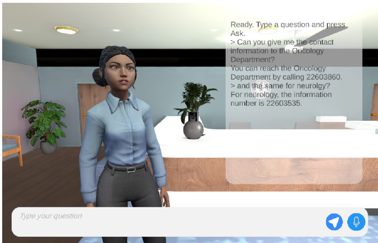
Figure 4.5: Example end-to-end interaction showing a follow-up query handled through the Unity frontend and answered using the backend retrieval pipeline.
