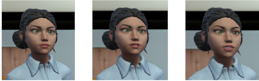
Figure 4.6: Avatar lip synchronization during speech playback, showing different mouth positions generated from audio-driven viseme animation.
