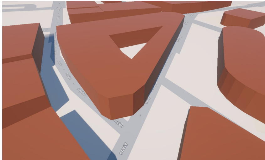
Figure 6.4: Unity building and road mismatch at Old Nicosia
