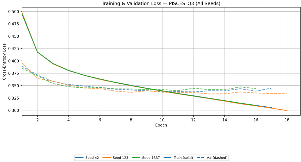
Figure 5.4. Training and Validation Cross-Entropy losses on 3-State of each of the three-models with randomly initialized weights (42, 123 and 1337), when trained on the 80/20 split of the PISCES dataset.
