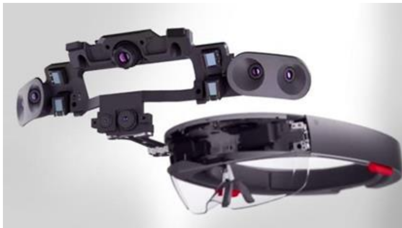
Figure 3.2 – HoloLens Sensors and Camera
