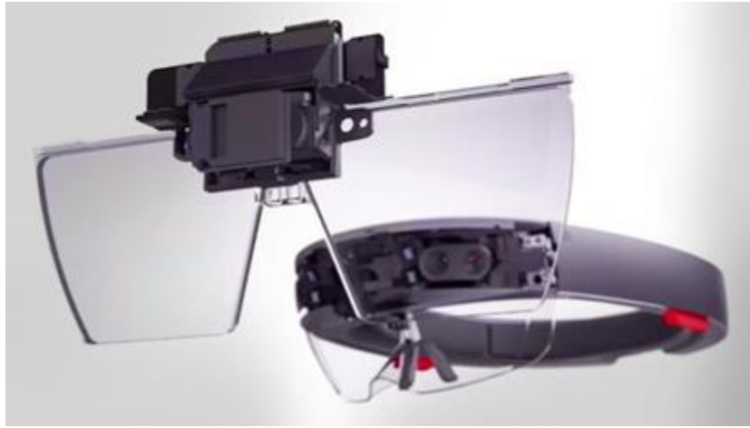
Figure 3.1 – HoloLens see-through lenses
