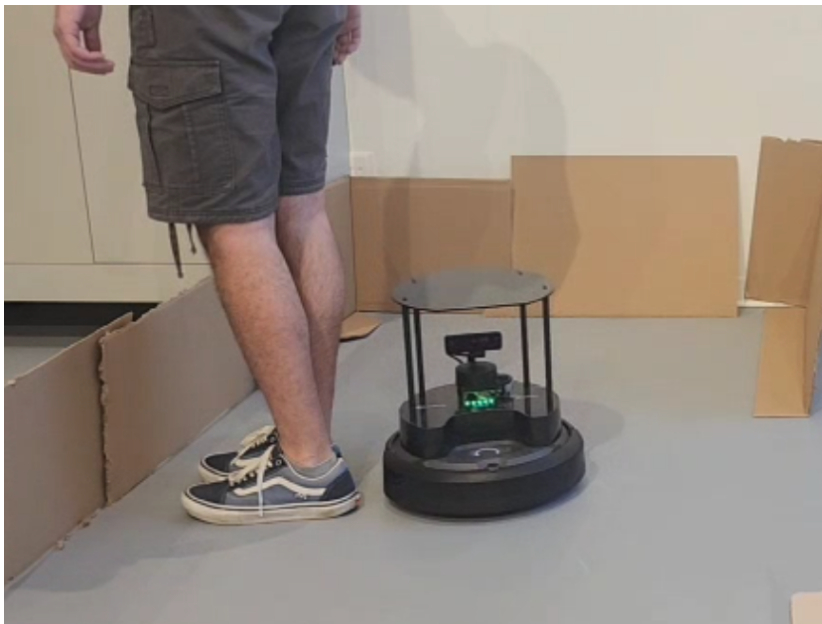
Figure 4.18: Scenario 6: The robot re-plans its route and moves around the human obstacle
