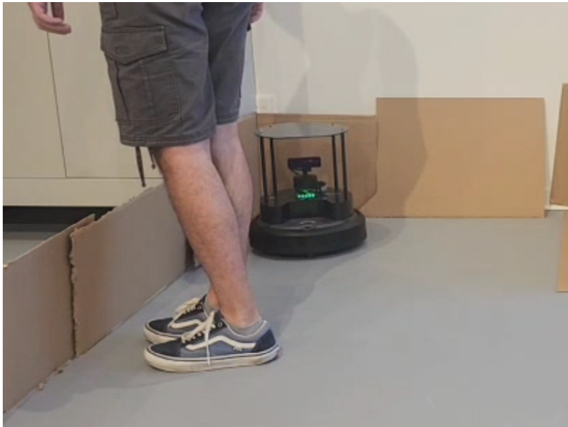
Figure 4.17: Scenario 6: The robot moves back after it detected a person
