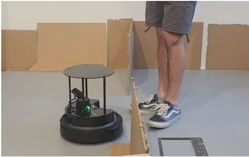
Figure 4.8: Scenario 3: The robot stops in front of the human obstacle
