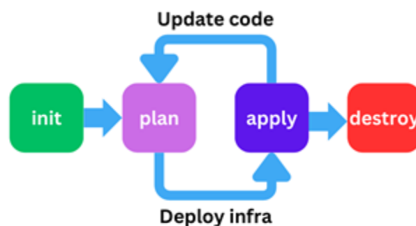
Figure 3.2.1.1: How Terraform works.
