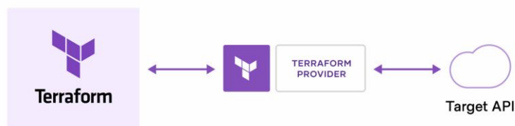
Figure 2.1.2.1: How Terraform Providers work.
