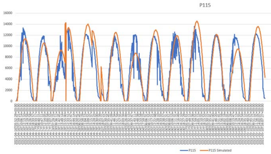
Figure 6, Chart comparing P115 Array located at UCY with the simulated P115 Array
