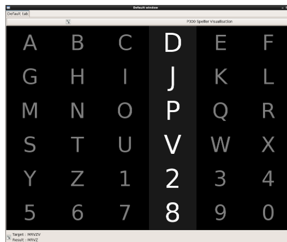
Figure 3-1: Basic Graphical User Interface of a modern P300 Spelling Device
