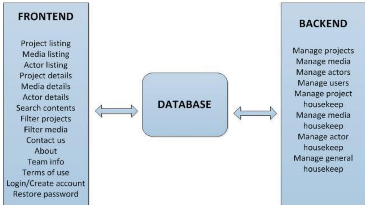
In the preceding figure the frontend and backend system components are presented. The frontend requests and retrieves data from the database for presentation purposes, and the backend requests and retrieves data from the database for management and storing purposes.
