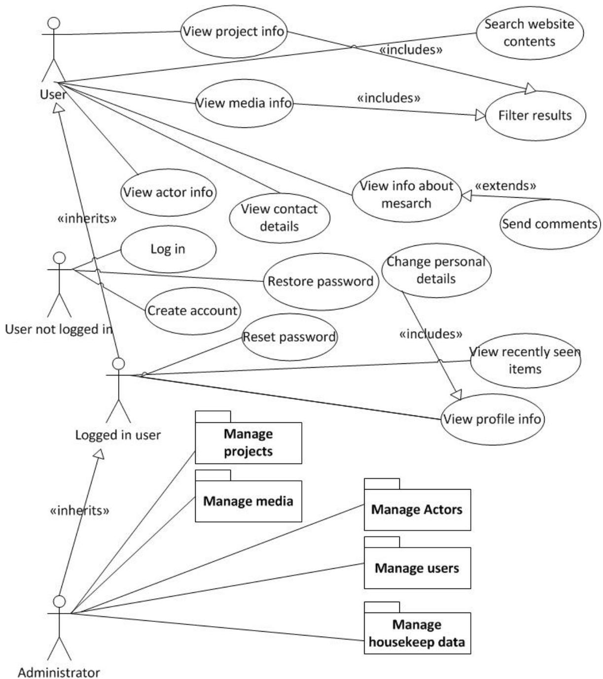
The preceding diagram describes the general functionalities of the system. Logged in and not logged in users both inherit user properties and additionally the administrator inherits the logged in user properties.
