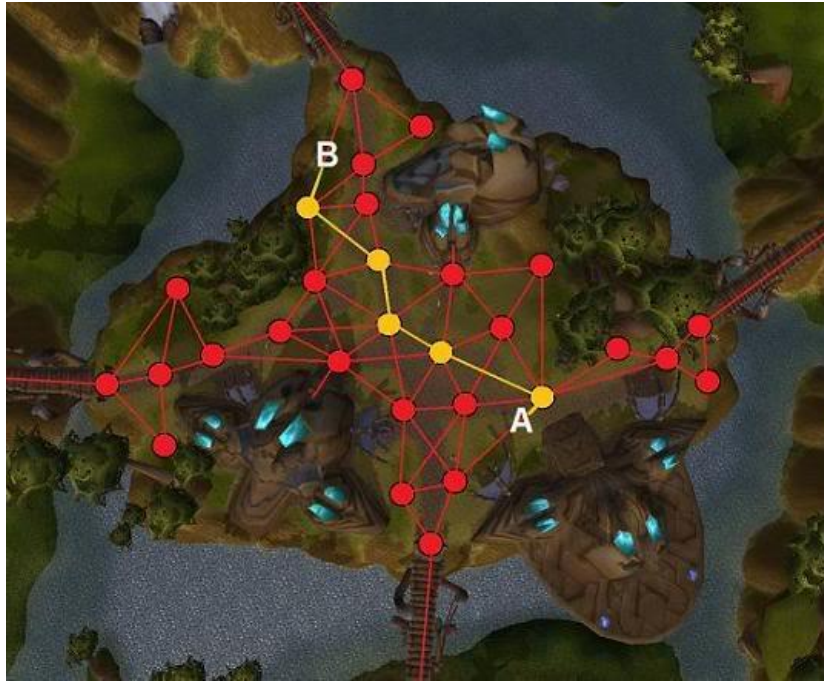
Figure 4-18: A waypoint graph in a scene in World of Warcraft game. Red dots stand for the nodes of the graph, while yellow ones indicate the shortest available path from node A to B. All lines are edges of the graph composing the various paths a kinematic agent could follow[28].
