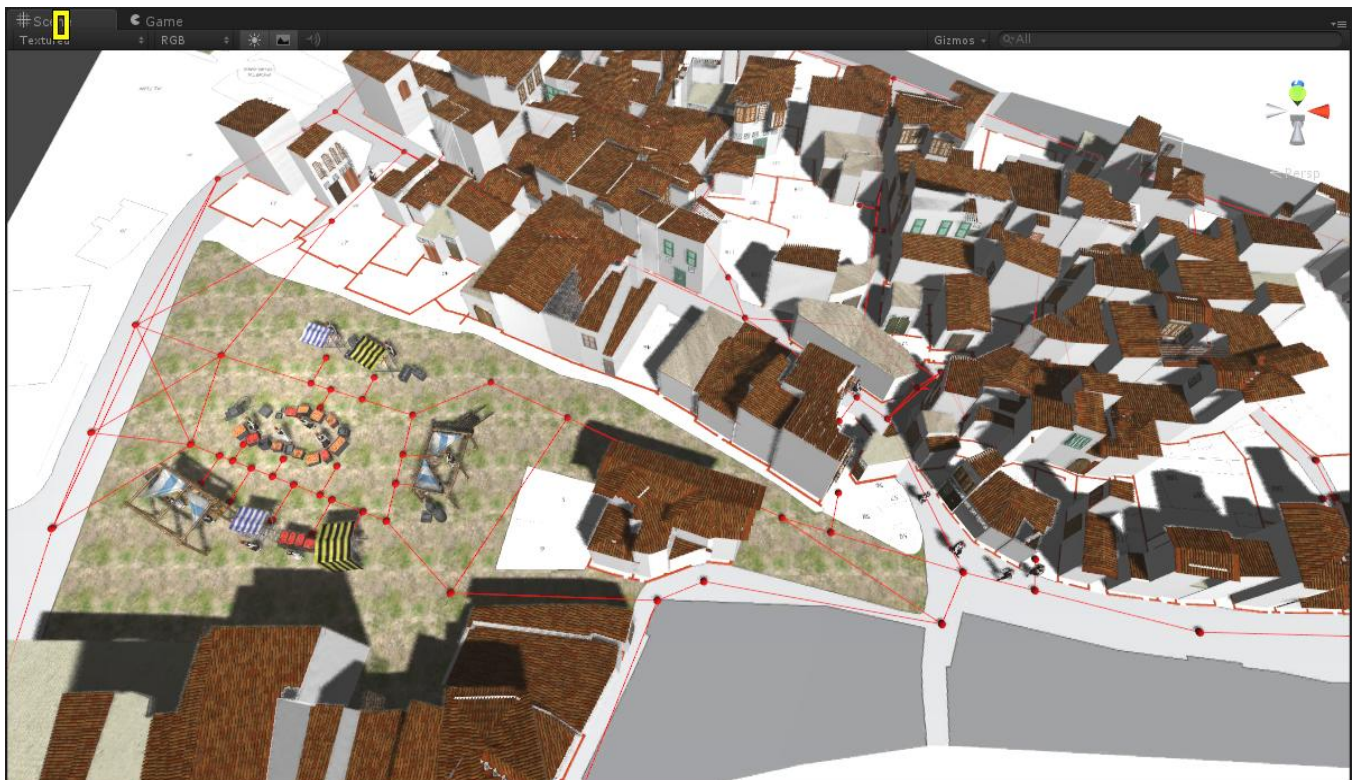
Figure 5-36: Graph produced is denoted in red. Small spheres show the position of nodes, while lines show the connections between the various junction nodes.
