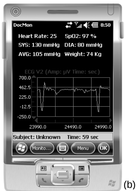
Fig. 2. (a) Snapshot of the PatMon module showing 12-ECG lead and SpO_2 signals locally at the patient's site. (b) Snapshot of the DocMon module showing 1-lead ECG transmitted to a windows mobile device. (c) Snapshot from the web interface of the CardiacPortal module, showing a waveform of 1-lead ECG retrieved from the central database. ECG analysis codings are shown at the lowest part of the screen.
