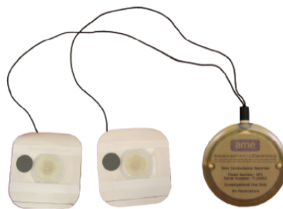
Figure 4: Wearable Skin Conductance Monitor / Recorder
