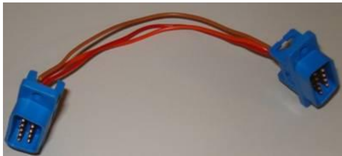
Σχήμα 6.23: custom – made καλώδιο RS232 male to RS232
