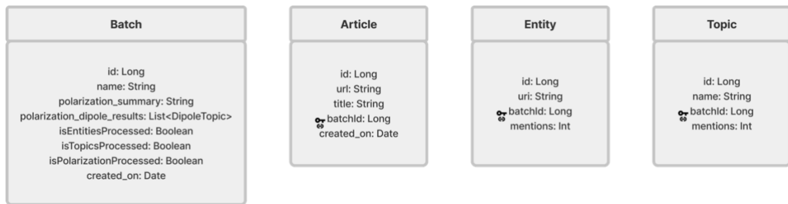
Figure 8 - Local Traditional SQL scema of Local Room Database of Android application showing four tables (Batch, Article, Entity, Topic) with their columns.
