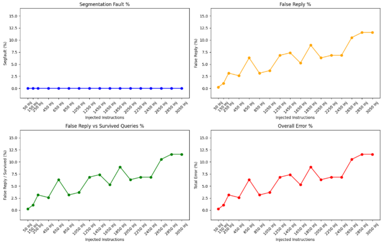
Figure 7.3 – Error behavior under increasing fault injections per query targeting floating point operations
