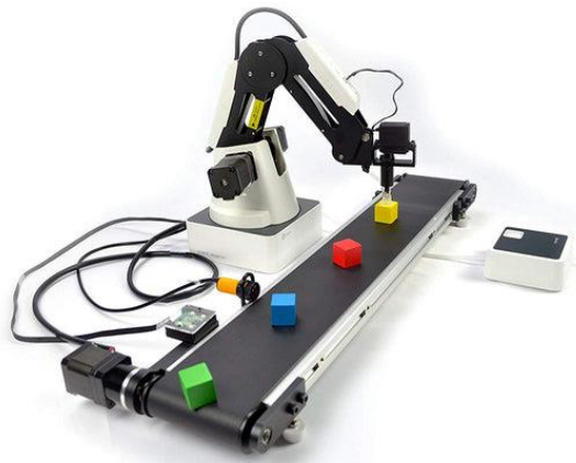
Figure 2.1 Dobot magician with the conveyer belt kit
