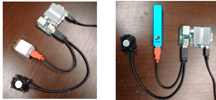
Image 2.5b: Connection to host and power through socket (left) and through powerbank (right)[13]
