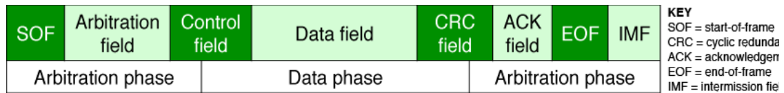
Figure 2-4 CAN Frame Structure [11]
