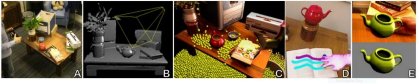
Figure 14: KinectFusion. A) user holding a Kinect. B) reconstructed 3D model with camera pose. C) texture-mapped model with simulated particles. D) touch interaction example. E) object segmentation (Izadi et al. 2011).
