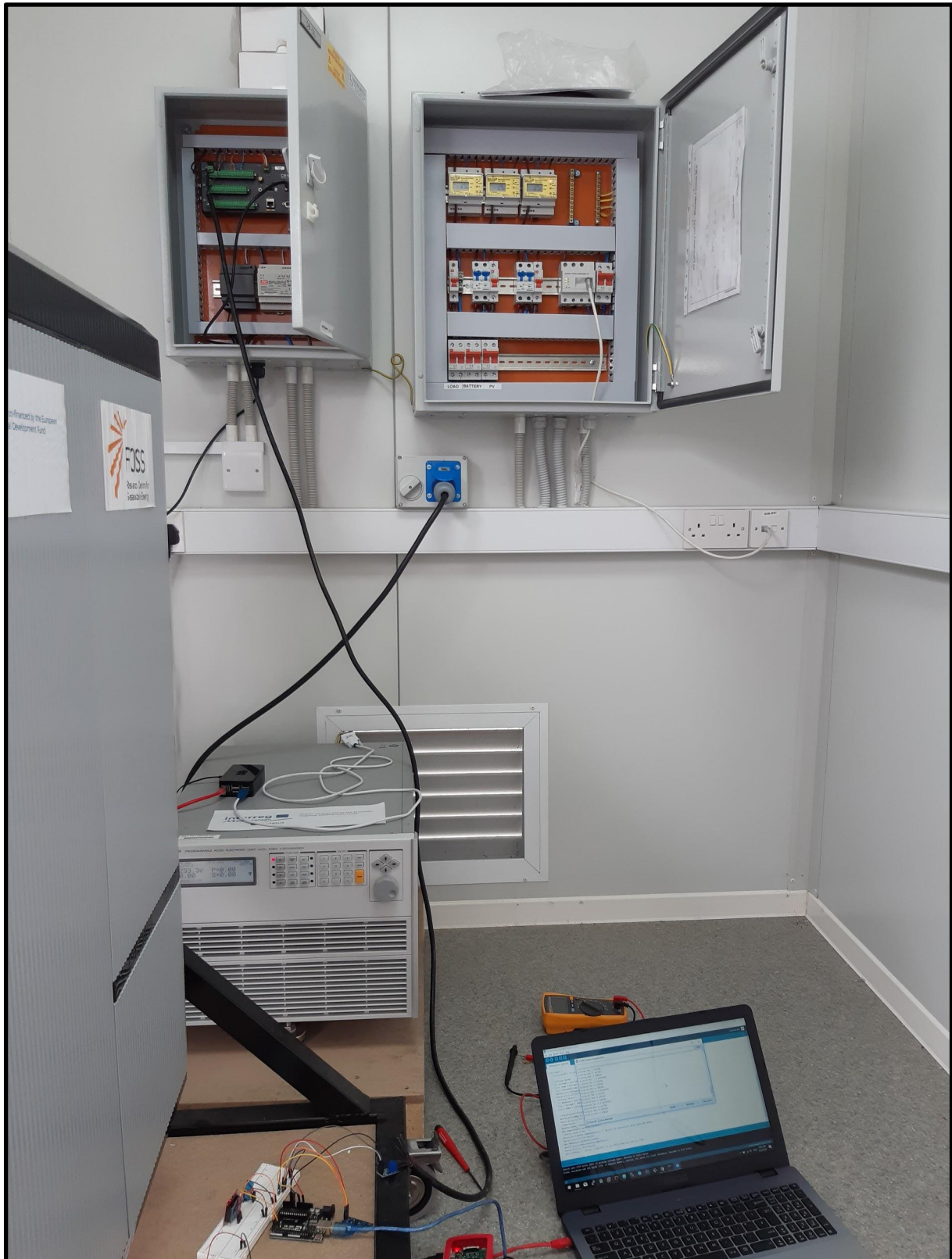
Image 1: Implementation of the apparatus at Foss Research Center. Data Logger can be seen inside the upper left white box.
