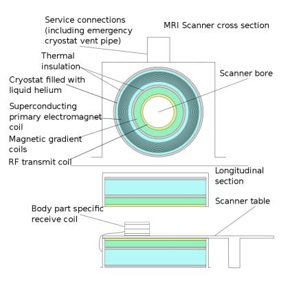
Fig 16. Detailed cross section of an MRI scanner.[13]
