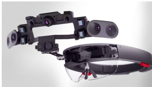
Figure 3.2 – HoloLens Sensors and Camera
