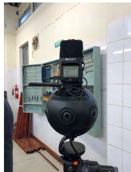
Figure 5.1 - Zoom H2n attached on top of the Insta360 Pro 2 with the Zoom H2n's interface
