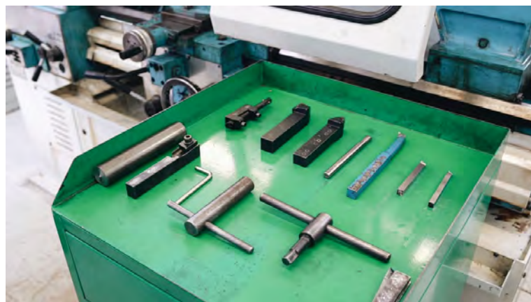
Figure 2.7 - Tools that are needed to operate the lathe machine
