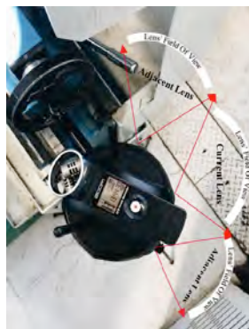
Figure 4.6 - Top View of the Insta360 Pro 2 and the field of view of each lens
