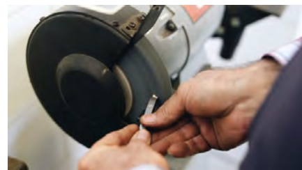
Figure 3.4 - Sharpening the tool
