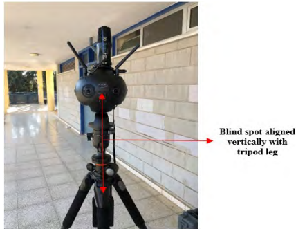
Figure 5.2 - Insta360 Pro 2 setup on a tripod to hide legs between blind spots
