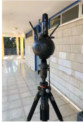
Figure 2.1 – Placement of Zoom H2n Recorder on top of the Insta360 Pro 2
