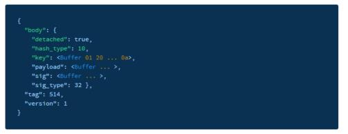
The packet is encoded using canonicalized msgpack and then standard Base-64.
