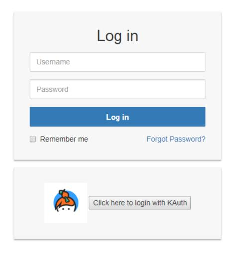
Figure 4.1: The login page offers the user the option to login using a username and password or to "Login with Keybase". Choosing to login with Keybase, the user is redirected to the Authorize controller of the OAuth server. This controller redirects the user to the login page of Keybase Website.
