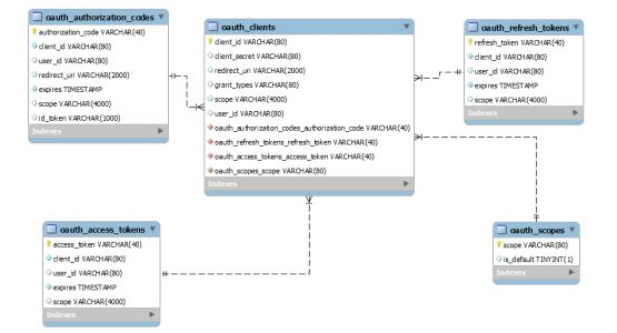
Figure 4.12: The database schema used for the OAuth2 server was instructed by the library we used.
