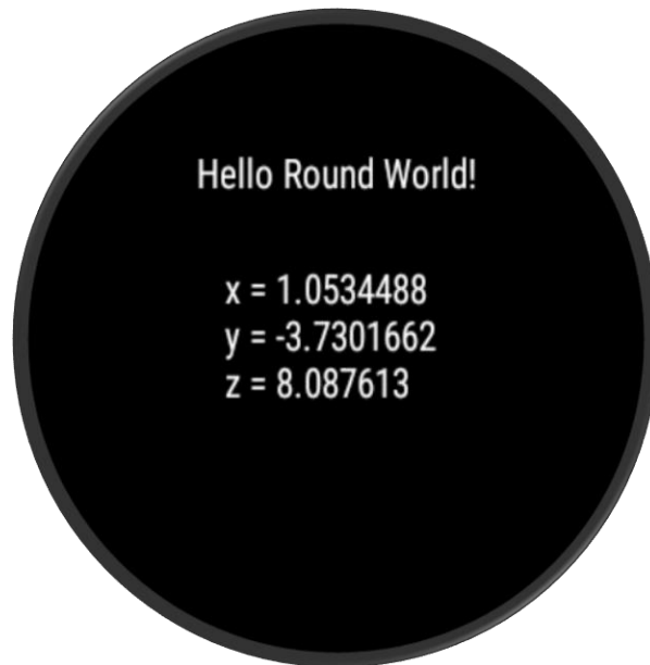
Figure 9. TestAppV1.0 Accelerometer data on wearable device
